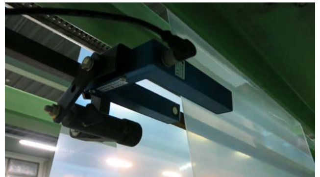
Ultrasonic Sensor DU-2 is used on clear film
